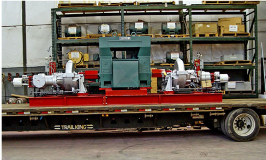
Dual turbine system ready for shipment from Turbosteam shop
