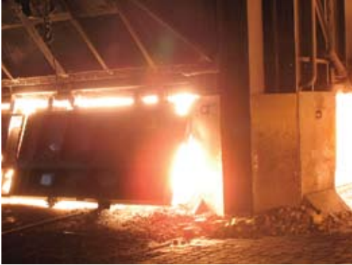
Electricity, coal and wood chips melt quartz in a large furnace where temperatures reach 3,000° F.
