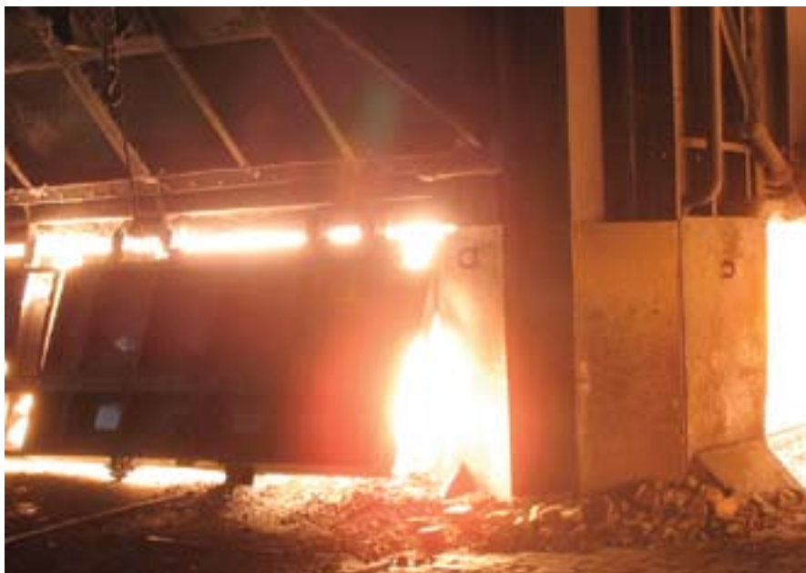
Figure 3. In a West Virginia plant, electricity, coal and wood chips melt quartz in a large furnace at temperatures around 3,000 degrees Fahrenheit, to produce silicon. The plant is undergoing a conversion process, to be completed in 2010, that will allow it to use much of its byproduct heat to generate power. The recycled heat can produce up to 45 megawatts of electricity, without burning any additional fuel. Image courtesy of Recycled Energy Development.
